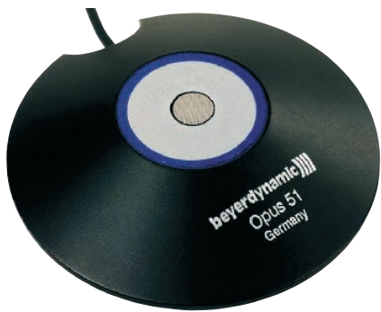
Boundary microphones, such as the Beyerdynamic Opus 51 pictured here, are often used in piano-recording applications because of their well-behaved hemispherical polar patterns, slim design, and comparative affordability.
