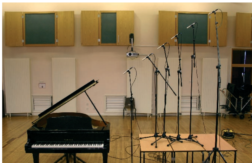
When creating an ambient recording of a piano, the distance of the microphone dictates to a great extent the ratio between the direct and reverberant sound levels captured. You can hear this in action in the 'Distance' audio examples, where six identical omni mics were set up at different distances from the centre of the piano, as shown in the picture.
